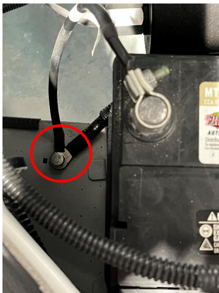
-Negative Chassis Ground Connection
