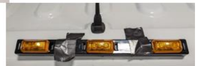
Temporarily tape lamp in place for making wire connections in cab
