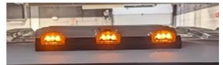
Tape off splices and check for operation of ID lamp
