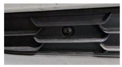
Locate and remove (3) Phillips head screws to remove grille. Gently pull-on grille to detach clips from cab.
