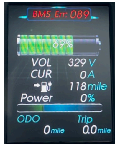
Figure 95: Example of a diagnostic trouble code “BMS_Err: 089”.
