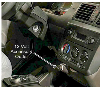
Figure 66: The accessory power outlet provides 12-volt power for accessories.
