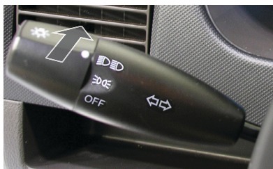
Figure 31: Push the lever forward to turn on high beams.
