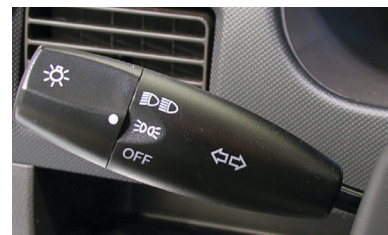
Figure 29: The lights are in the running lights position.
