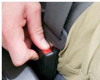
Figure 13: Press the red button to unfasten the belt.
