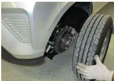
Figure 83: Remove the tire.
