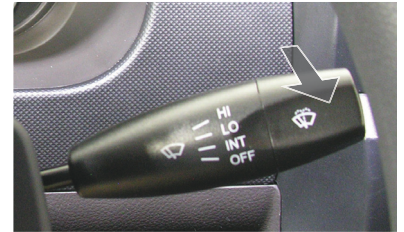
Figure 35: Pull the lever back to spray washer fluid.
