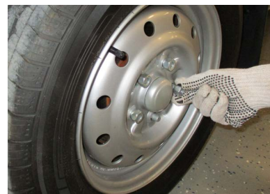
Figure 87: Install the wheel lug nuts by hand, leaving them finger tight.
