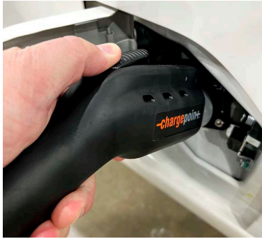
Figure 4: Insert the charging plug into the charging port.
