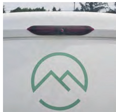
Figure 63: The backup camera is built into the center high mounted stop lamp.
