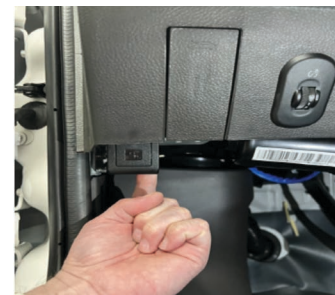
Figure 2: Charging port door release handle.
