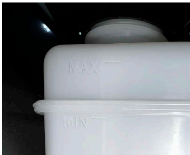
Figure 89: Brake fluid reservoir minimum and maximum fill levels
