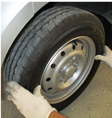
Figure 86: Place the wheel over the wheel studs.
