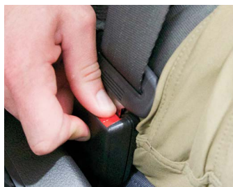
Figure 13: Press the red button to unfasten the belt.
