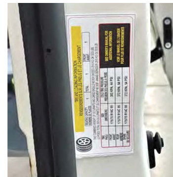
Figure 18: The tire pressure placard is located in the driver's door frame.
