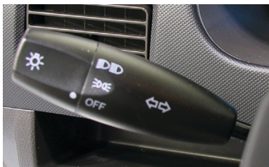
Figure 28: The lights are in the off position.
