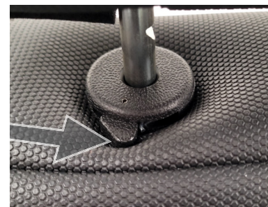
Figure 17: Pressing the lock button allows lowering, or removal, of the head restraint.
