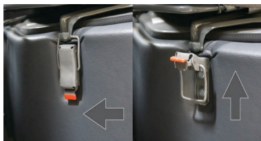
Figure 61: Latch secured-left, latch released-right
