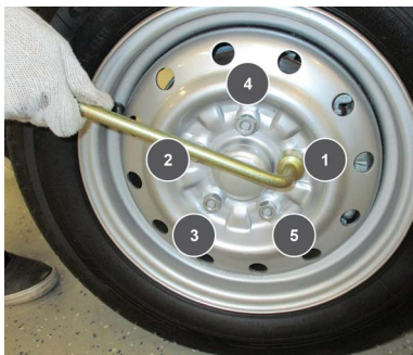
Figure 88: Tighten the wheel lug nuts in a star pattern as shown from 1 to 5 above.
