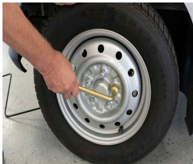
Figure 78: Loosen the wheel lug nuts before lifting the wheel off the ground.
