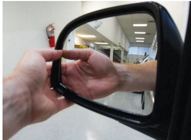
Figure 62: Adjust the glass mirror inside the housing.
