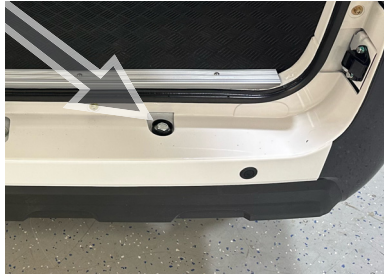
Figure 75: Use the lug wrench to lower and release the cage that supports the spare.
