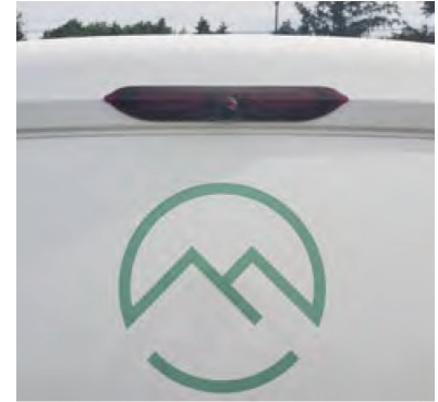
Figure 63: The backup camera is built into the center high mounted stop lamp.
