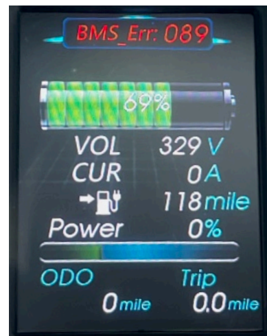
Figure 95: Example of a diagnostic trouble code “BMS_Err: 089”.
