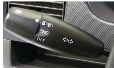
Figure 30: The lights are in the on position.
