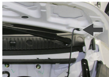
Figure 11: The hood support rod secures the hood in the open position.
