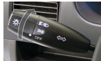
Figure 27: Turn the knob to control the lights.
