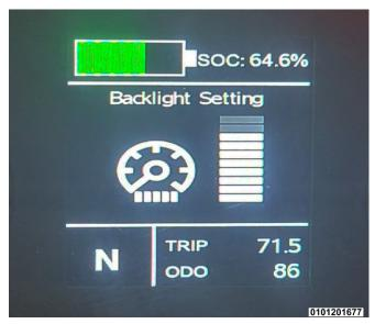
The backlight setting allows the driver to adjust the amount of illumination in the display screen. Press and hold the TRIP button to change lighting settings once at the Backlight screen. The backlight setting will work when the light switch is in the ON position.
