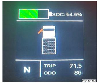
This screen display shows the status of the doors, open or closed or if either of the cab doors are not securely closed on the vehicle.
