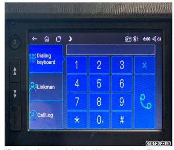
When a phone is connected with the vehicle you can make a call by entering a number in the touchscreen radio keyboard. To manually type in a phone number, use the Dialing keyboard. Enter the number and press the phone symbol to activate the call.
