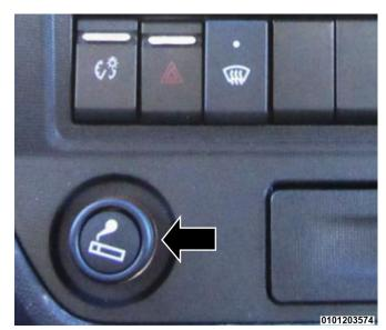
The cigarette lighter is located in the instrument panel to the right of the steering wheel and next to the ashtray. To activate the cigarette lighter, push in on the warming socket of the cigarette lighter in the instrument panel. When the socket is heated it will automatically pop up from the depressed position, the surface of hot lighter will be red. When it is red, it is hot and ready for use.
