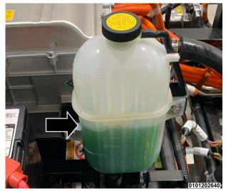
**High Voltage Battery Coolant Reservoir**
