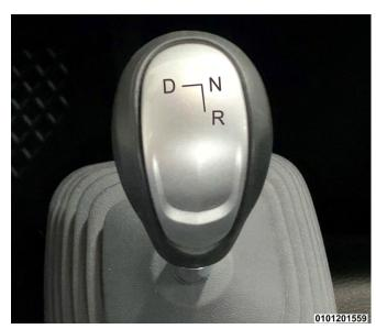
The gear shift selector is used to shift between the driving gears DRIVE (D), NEUTRAL (N), or REVERSE (R). The vehicle must be in the NEUTRAL (N) position before you can start the vehicle. Apply the brakes before shifting into any driving gear.
