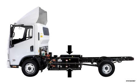
The high voltage batteries are located behind the cab on each side of the vehicle frame.
