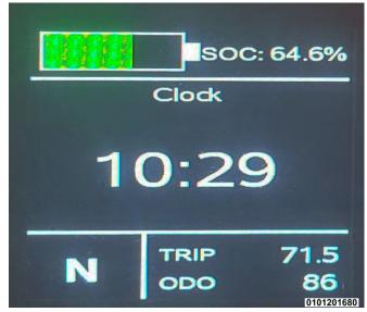
The clock screen displays the time and allows you to update the time from the TRIP button on the multifunction lever.
