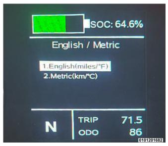
The English/Metric setting allows the driver to select the type of measurement standard displayed on the cluster, such as Miles/Kilometers or Fahrenheit/Celsius preferences. Once at the screen press and hold the TRIP button on the end of the multifunction lever, to switch between English/Metric choices.
