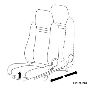
Pull up on the bar under the front seat to release the slide mechanism so the seat can slide backward or forward. Release the bar after reaching the desired position so that the seat base will lock into position securely. The seats can slide forward and rearward to adjust the seat to properly operate the brake and accelerator pedals.
