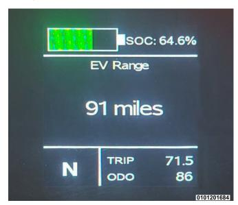
The EV Range screen tells approximately how many miles are remaining on a charge.
