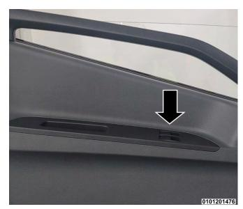
The driver's and passenger's side windows can both be opened or closed from the dual switches on the driver's door. The passenger can open or close their window using the single switch on the passenger side.
