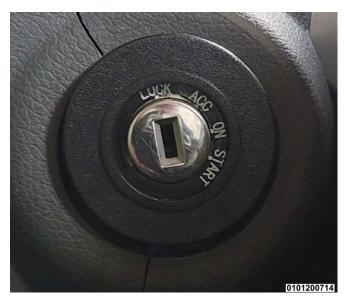
**LOCK** — The key can be inserted and removed from this position. You can cycle the key from the lock position through the other positions.
