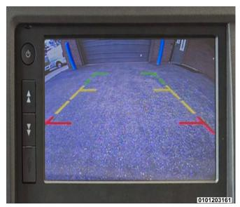
A backup camera may be installed on the rear of the vehicle. The camera will automatically turn on whenever the vehicle is shifted into REVERSE (R). The camera will display the view behind the vehicle on your radio screen. The camera display will turn off when the vehicle is shifted out of REVERSE (R).
