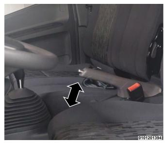
To engage the parking brake, pull up firmly on the parking brake lever. To release the parking brake, push the button on the end of the parking brake lever, lift up slightly and lower fully to disengage.
