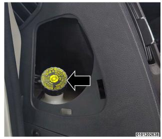
The brake fluid reservoir access panel is located on the driver's side of the instrument panel, near the door frame.
