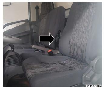
Pull the lever on the side of the center seat back, to fold the center seat back down flat. The back of the center seating position has cup holders when the seat back is folded flat. To raise the center seat back, lift up on the lever and fold the seat back to the upright position until it is secured in place.
