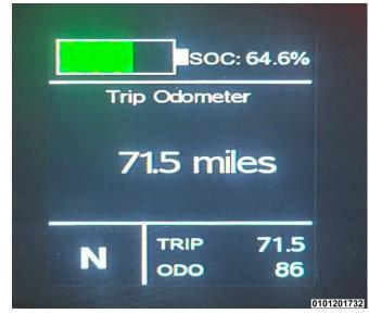
The trip odometer will measure the distance traveled on a trip. The driver can press and hold the TRIP button on the end of the multifunction lever to reset the trip odometer back to zero.
