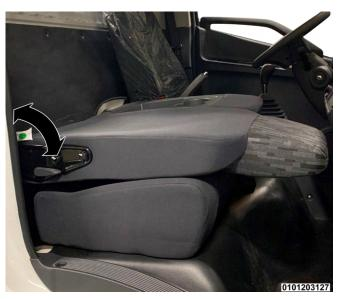
To fold the outboard passenger seat flat, pull the lever on the outside edge of the seat back. To raise the outboard seat back, lift up on the lever and fold the seat back to the upright position and secured in place.
