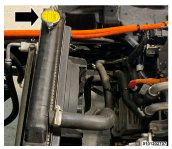
**Drive Motor Cooling System Radiator**
