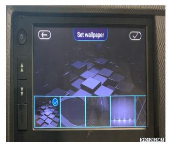
Press the back arrow in the upper left corner of the display screen to return to the "Settings" screen.
