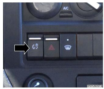
When the headlights are on, the brightness of the radio, instrument panel switches, steering wheel controls, and climate control dials can be adjusted. Press it once for brighter, press it again for dimmer.
