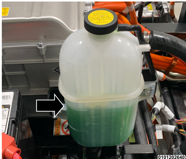
High Voltage Battery Coolant Reservoir
