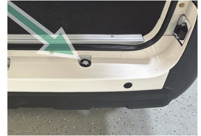
Figure 49: Use the lug wrench to lower and release the cage that supports the spare.
