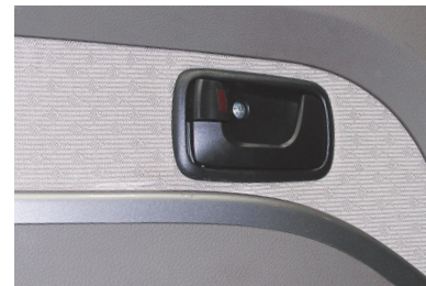
Figure 8: The door lock is located with the door handle. When the red indicator shows, the door is unlocked.
