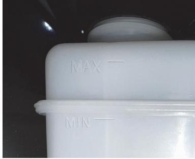
Figure 61: Brake fluid reservoir minimum and maximum fill levels
