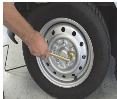
Figure 52: Loosen the wheel lug nuts before lifting the wheel off the ground.
