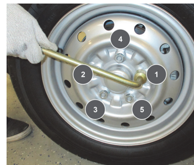
Figure 59: Tighten the wheel lug nuts in a star pattern.
