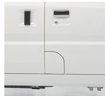
Figure 1: The charging port door is located at the lower-left corner of the front passenger door.
