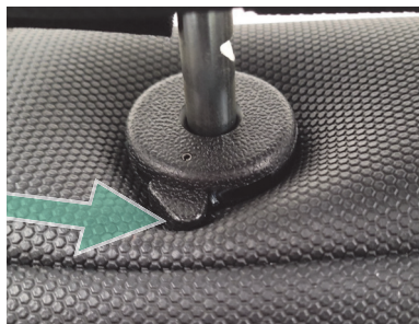
Figure 41: Pressing the lock button allows lowering, or removal, of the head restraint.
