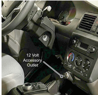
Figure 43: The accessory power outlet provides 12-volt power for accessories.
