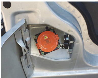
Figure 2: To provide access to the charging port, the charging port door is opened by pulling a handle at the driver's position.
