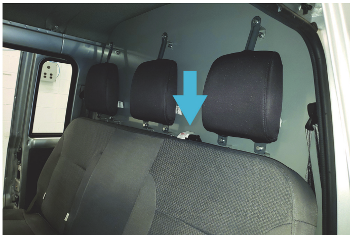
Figure 39: Head restraints help protect the neck in the event of a collision.
