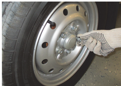
Figure 58: Install the wheel lug nuts by hand, leaving them finger tight.
