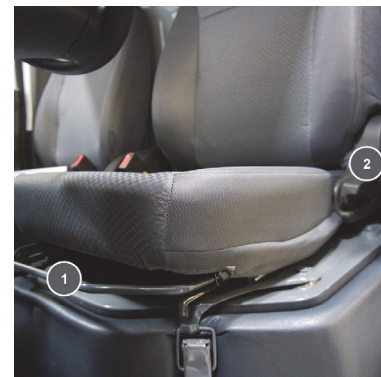
Figure 37: 1) Fore/aft lever. 2) Recliner lever
