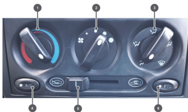
Figure 34: Cabin climate controls
