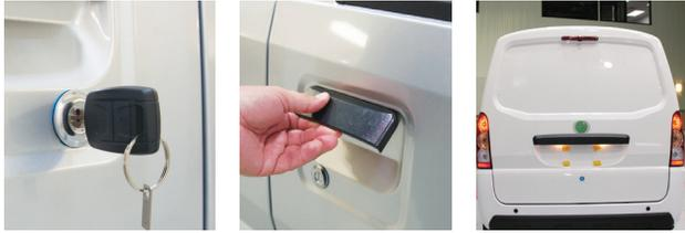
Each vehicle is equipped with two remote entry key fobs. The key fobs unlock/lock the doors and liftgate remotely.
