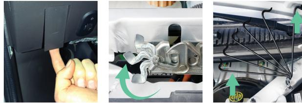
1. Locate the hood release on the lower left of the instrument panel.
