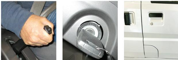
1. Before charging the vehicle, engage the parking brake, turn the key to the LOCK position, and remove the key.
